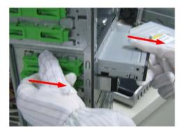
**5.** Release the rail and remove the Card Reader.
